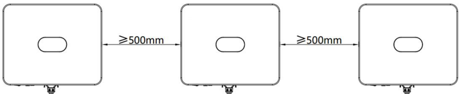
Fig. 4.5 Installation Dimension of Side-by-side Inverters
